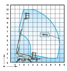
Max. working height 12.00 m Max. platform height 10.00 m Max. outreach 7.90 m Support width 3.15 / 3.55 m Lifting capacity 130 kg Basket size 0.75 x 0.80 m Boom rotation cont. Boom control 2-speed Transport length 5.52 m Transport width 1.72 m Transport height 1.96 m Weight 1390 kg Driving system std AC socket in the basket x 2 Batteries 140 Ah std DC Motor std Gradeability 25 %
